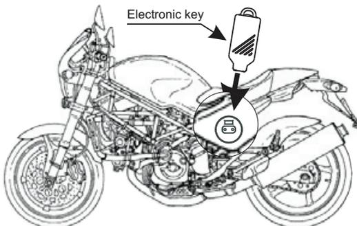
Example of receptacle positioning on the vehicle plastic fairing.
