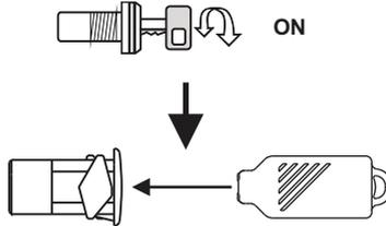
Two acoustic signals (a high and a low-pitch sound) and two flashes of the turn indicators confirm that the system is in programming mode.
