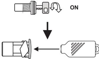
Two audio signals (a high and a low-pitched sound) and two flashes of the turn indicators will indicate that the system has entered the programming procedure.
